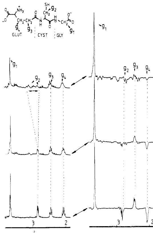
Figure 6. Titration of glutathione (0.033 M) with myocrisin solution (0.025 M) (a) in the standard FT NMR made and (b) in the spin-echo mode.
